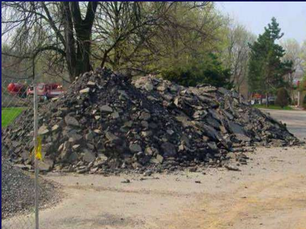
Broken asphalt reused as gravel base
